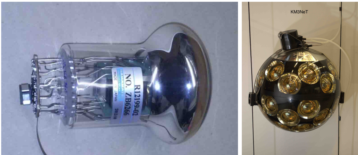
Figure 3.2.: Photos of a a prototype of a Hamamatsu photomultiplier (PMT) on the left, and a KM3NeT digital optical module (DOM) on the right [36]. 31 PMTs are installed in each DOM, visible as the golden disks.
