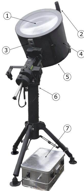
Figure 26: Image of DesertACT’s telescope body, showing 1: Fresnel lens (behind protective glass), 2: optional guiding camera, 3: 3” prism bar for telescope mount connection, 4: light shielding, 5: bottom flange (camera box not shown), 6: telescope mount, 7: power supply and auxiliary electronics.
