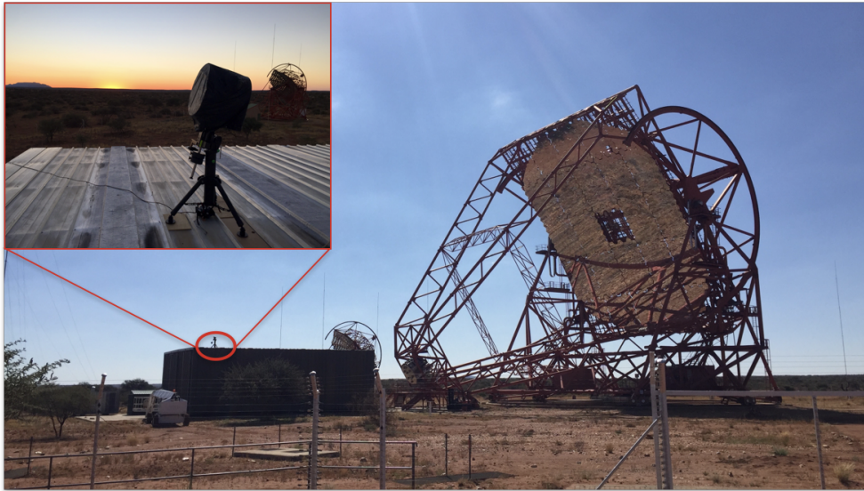
Figure 27: Photograph of the DesertACT setup on the instrument container close to the H.E.S.S. array centre during the Namibia campaign. A zoomed-in view of the DesertACT setup is also shown. The images are provided by Funk (2021).
