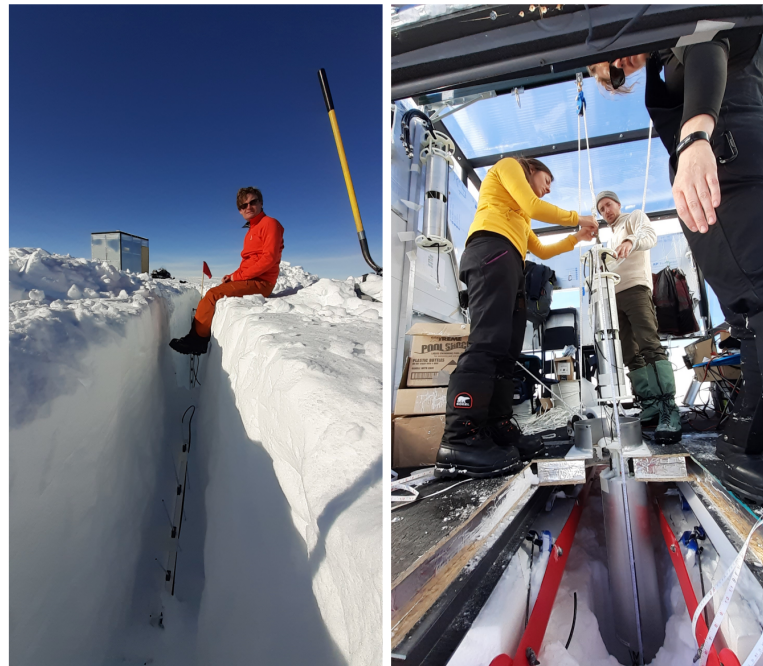
Figure 2: Antenna deployment. Surface antennas deployed in shallow trenches, deep antennas lowered into boreholes. Figure adapted from [16]
