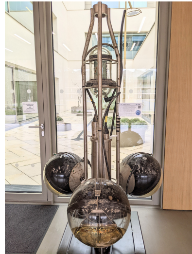
(B) An Optical Module Frame (OMF) from the ANTARES telescope. Now, an exhibition piece at ECAP.
