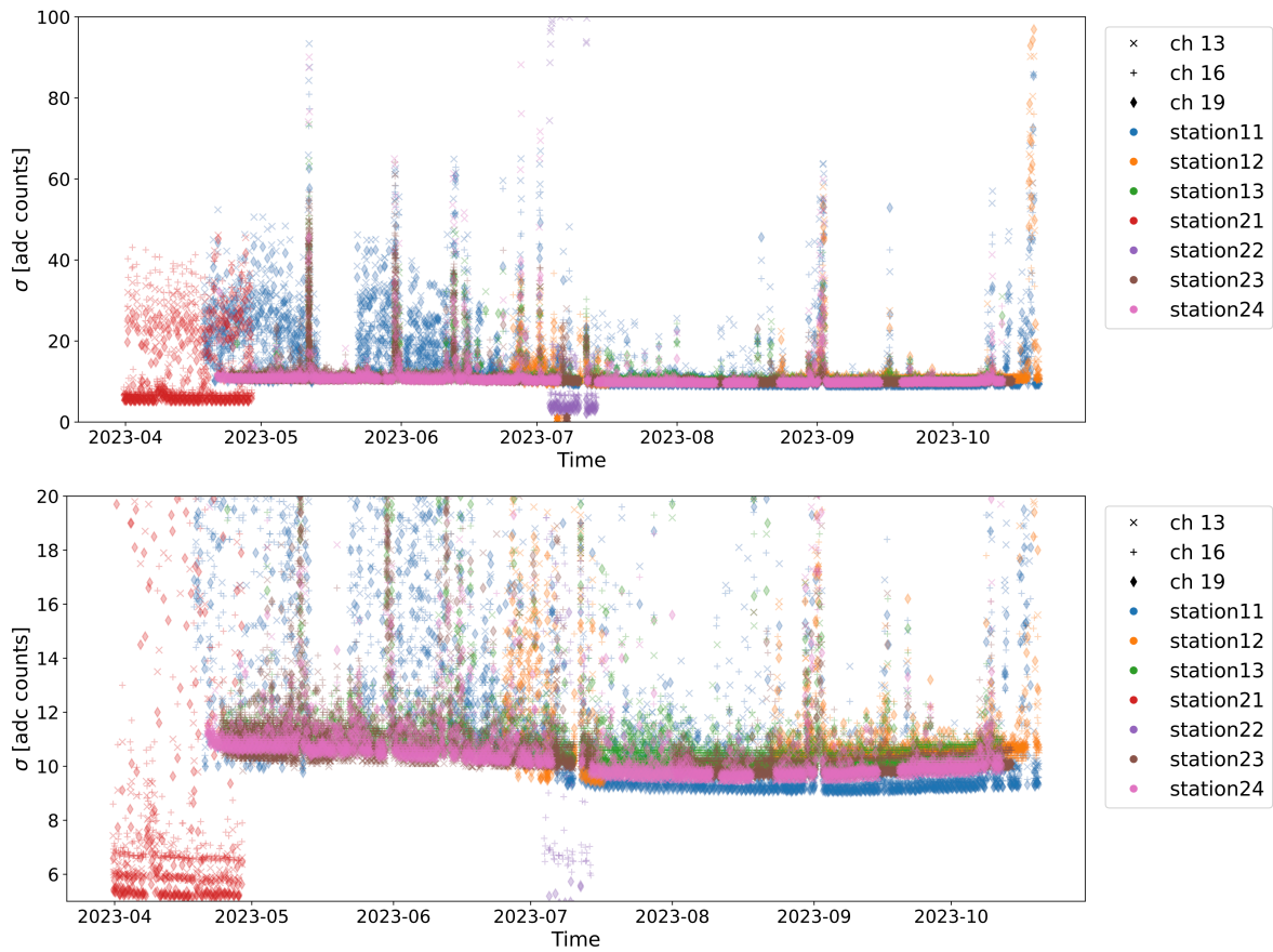
Figure 6.9: Overview of the \sigma_{\text{adc}} per run ( \sim 2 hours) in adc counts with baseline correction. About 10 000 events are shown for the 2023 season for all stations and the three upward facing LPDAs. The data is the burn sample transmitted via satellite for monitoring. All trigger types are considered. Top: \sigma in the range of 0 adc counts to 100 adc counts. Bottom: Same data but zoomed in.
