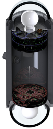
Figure 9: The POCAM used in the IceCube Upgrade. The laser of the POCAM will be modified into a fan beam to serve as the LOMlogger emitter [24].
