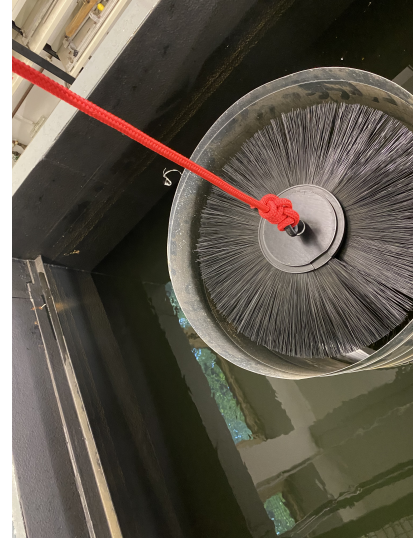
(b) Picture of the baffle being lowered into the pipe that simulates the borehole.
