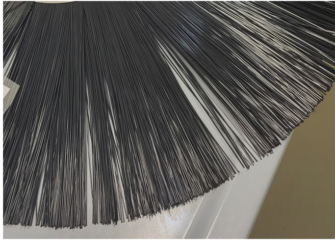
Figure 13: The image highlights a part of the baffle, where the bunching of the bristles is pronounced.
