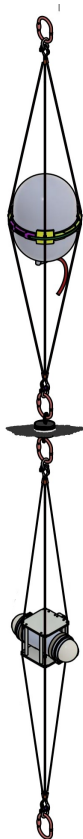
Figure 7: 3D-model of the LOMlogger. The LOM at the top, the baffle in between, and the POCAM at the bottom. The distance between LOM and POCAM is 2 m. The LOM is used as the detector of the LOMlogger and the POCAM as the source [19].
