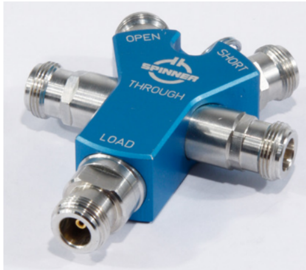
Figure 5: A manual calibration kit provides several types of line terminations required during manual calibration. [20]
