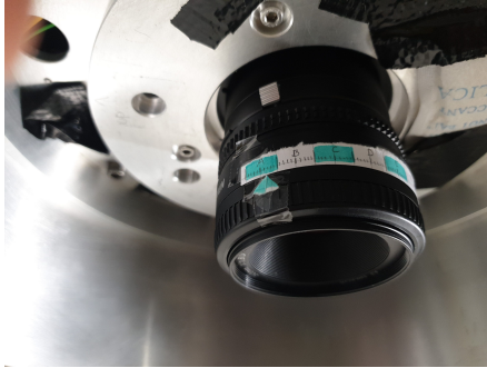
(a) The camera is focused with help of a handmade but sufficient scale to make objective settings easier comparable.
