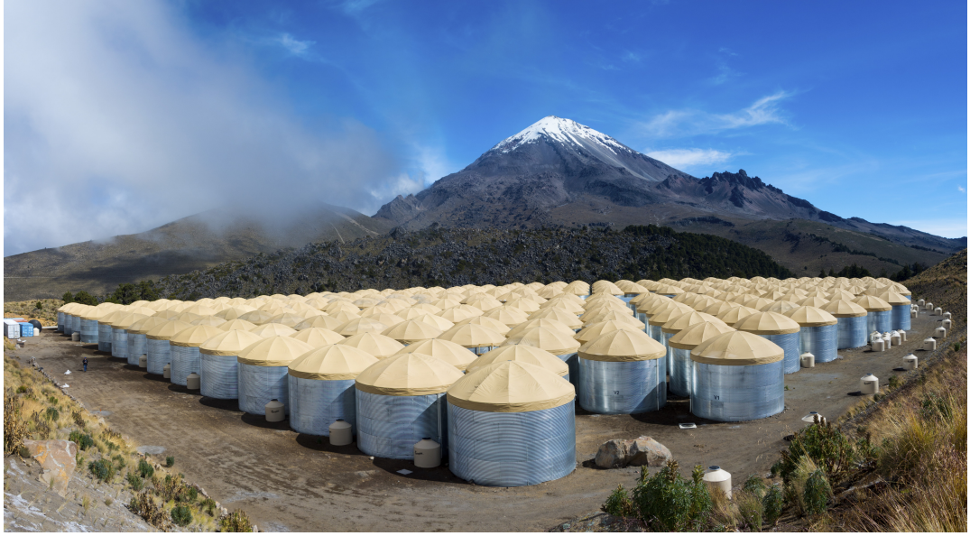
Figure 2.8: Photograph of the HAWC detector. We can see the array of steel water tanks in the middle. In the background the highest mountain in Mexico, the Pico de Orizaba. Taken from [43].
