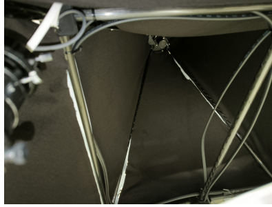
(b) View inside a MI 2 SO telescope, exposing the secondary stabilization frame, heating cables and closed off optics and detector tubing.
