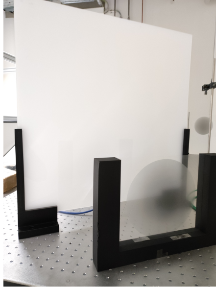
Figure 12: Transparent film with greyscale light intensity distribution printed on and plexiglass screen inside 3D-printed holding frames.
