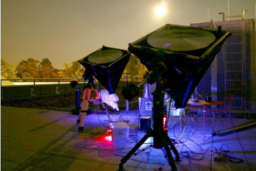
Figure 21: MI 2 SO in operation on the roof of ECAP observing Vega at high altitude. The black cloth tubing to block stray light such as from the moon (above one of the telescopes in the image) or artificial sources can be seen.
