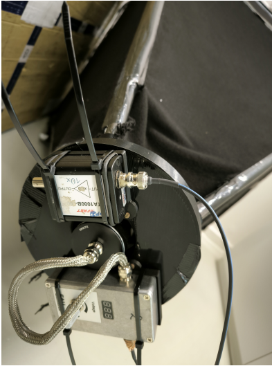
(c) PMT housing crown with PMT, gain control box and amplifier box.
