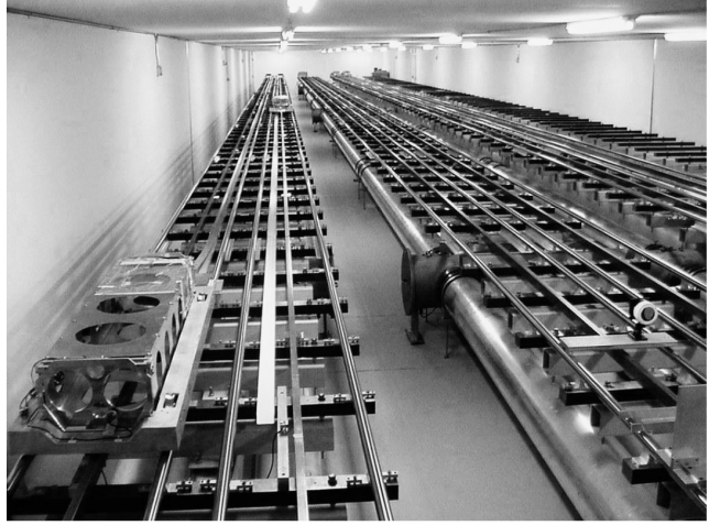
Figure 2.9: Left: geometry for two-telescope interferometry. The image is adapted from [49] with the violet text added. Right: delay lines for optical path length compensation for the CHARA array. Taken from [50].
