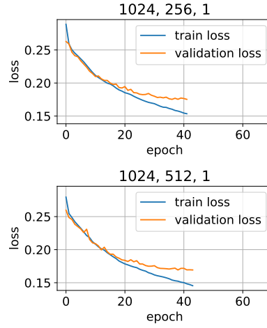
Figure 38: These are the learning curves of a RNN with a FC layer size of 1024. The three numbers in the plot titles represent the FC layer size, the size of the LSTM layer and the number of LSTM layers.
