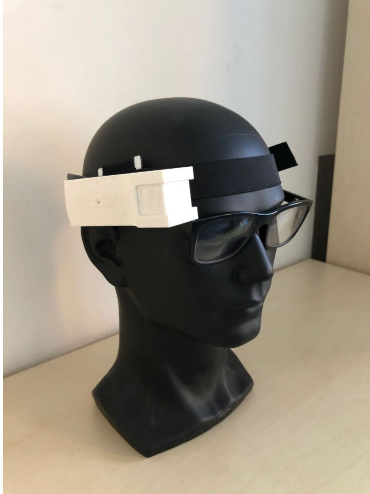
Figure 4.26.: Prototype of the H_p(3) dosimeter with one Dosepix detector. The case material consists of white photopolymer resin. The notches in the cover indicate the position for lead glass filters. Those filters will resemble the attenuation of radiation protection glasses worn by the user. The prototype is fixed to a headband which is attached to the head of the user. The position of the sensor element of Dosepix is as close to the eye as possible. The normal vector of the sensor element is parallel to the viewing direction of the user, i.e., the dosimeter looks in forward direction.
