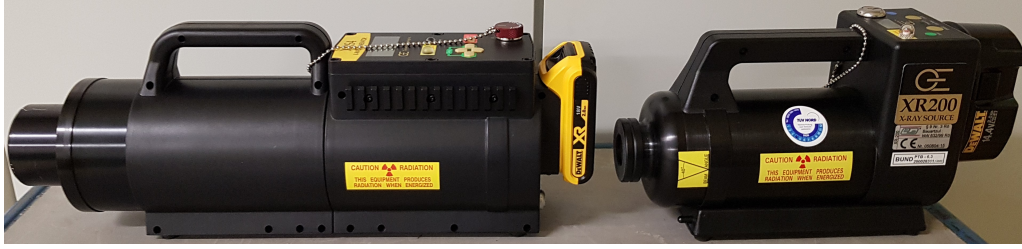
Figure 8.1 Photograph of the two X-ray generators the measurements are performed with. Left: XRS4 [60], right: XR200 [61].
