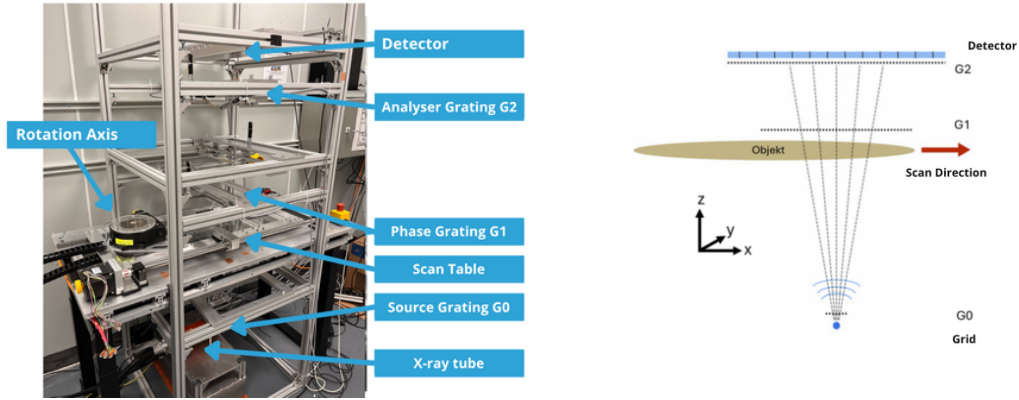
Figure 39: (Left) A photograph of the scanner setup is shown. The orange X-ray tube is located in the lower part of the image, above which is the G0. The scanning table is located between the G0 and the G1 and is moved horizontally during the scan, above which the rotation controller is put. The G2 is positioned at approximately a fractional Talbot distance from G1. Above that, there is a detector 1385 mm away from the source. (Right) Schematic representation of the scanner setup. The scanning direction is the x-direction. The grating, detector, and object table are in the x-y plane. The lattice bars are oriented along the y-axis. The optical axis runs in the z-direction. Image taken from [32].
