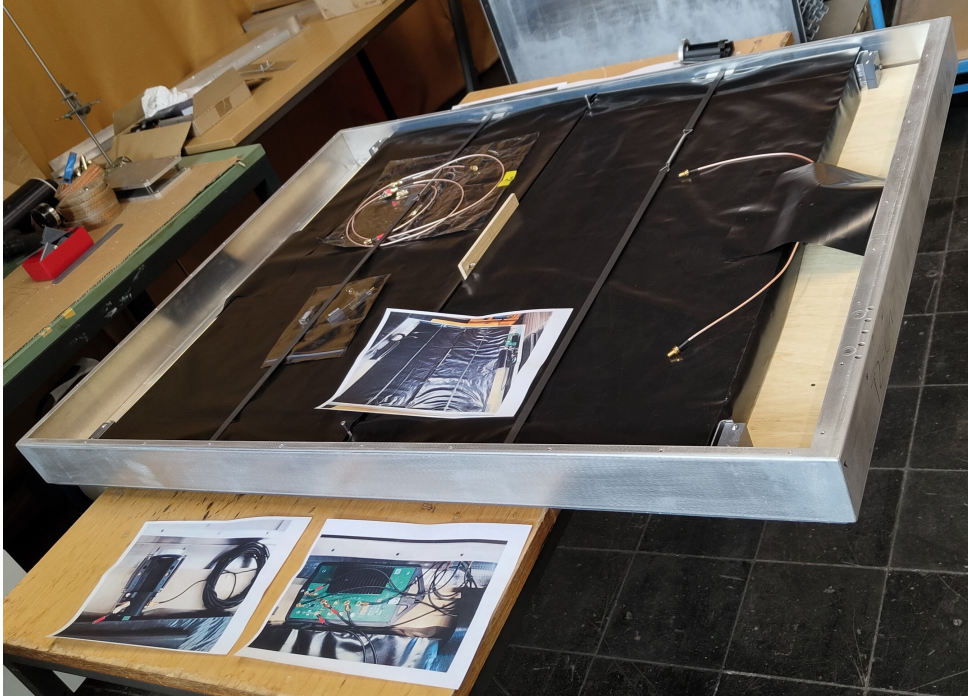
Figure 3.4: Photograph taken at the Karlsruhe Institute of Technology (KIT), Germany. It shows a plastic scintillator module originally used in the KASCADE-Grande experiment [24]. These scintillators have been repurposed for use in current projects such as LORA (LOfar Radboud Air shower array). They are also intended for future applications, such as the Muon Tower component of the Square Kilometre Array (SKA), which will be the world's largest radio telescope [4].
