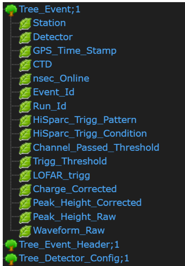
Figure B.2: Structure of the Tree_Event in the new ROOT data format. Unlike the old ROOT structure, the new ROOT structure does not comprise of Det1, Det2,...Det20.
