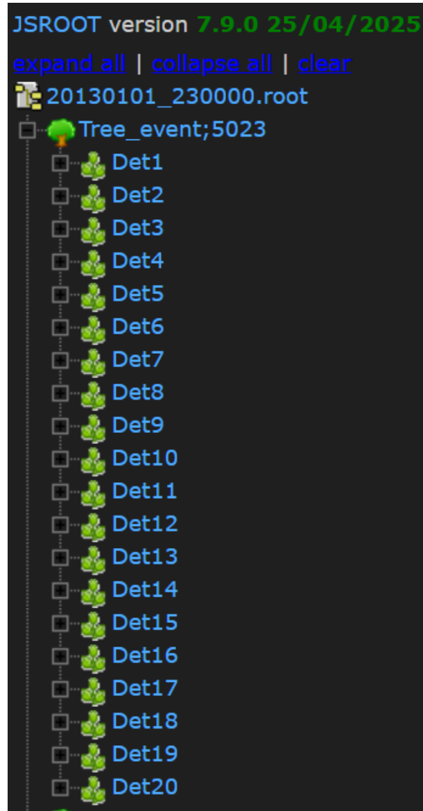
Figure B.1: Structure of the Tree_event in the old ROOT data format. Each detector (Det1 to Det20) is represented as a separate branch containing subfields such as GPS timestamps and detector-specific measurements.[38]
