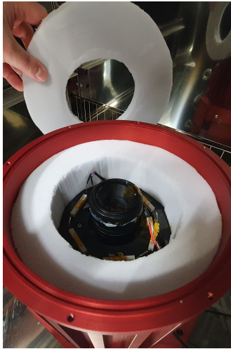
Figure 16: Initial resistor insulation setup (referred to as ring insulation ), with upper ring to be placed on top of lower ring.
