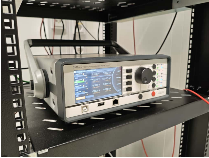
Figure 3.4: iseg SHR high-voltage supply used for PMT biasing.
