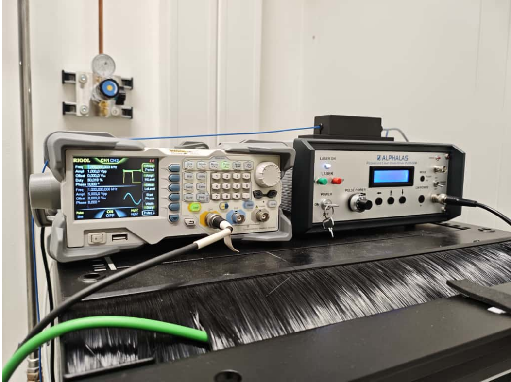
Figure 3.6: Signal generation: Rigol DG1022 gating the Alphas PLDD-50MHV pulsed driver.
