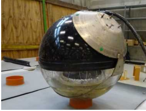
(a) ANTARES PMT before extraction
