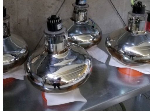
(b) ANTARES PMTs after extraction
