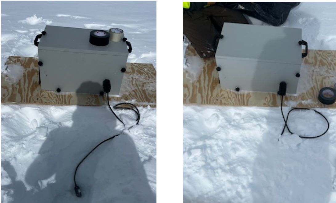
Figure 37: Deployment of the acoustic noise measuring equipment. The enclosure is placed on a wooden plank on the surface, while the glaciophone is buried in snow at a depth of about 0.5 m. Picture taken by Felix Schlüter.
