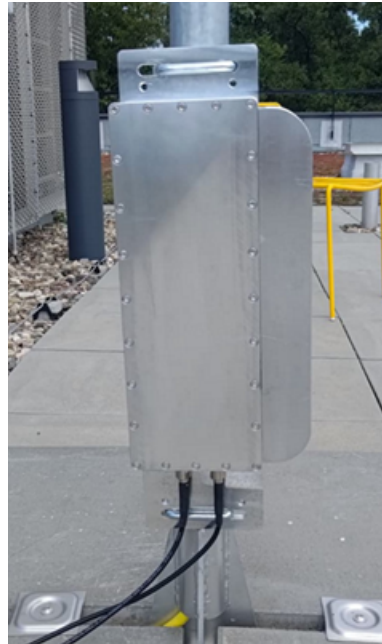
Figure 18: The divert load used at the ECAP-Station. The same device is used at the RNO-G detector stations.
