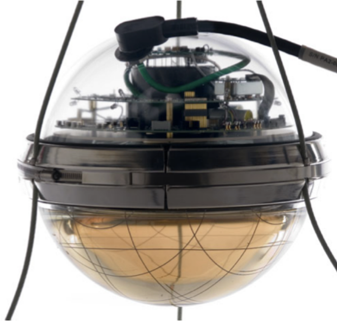
Figure 3.1: Picture of a DOM used in IceCube. The PMT in the lower hemisphere faces downward while the electronics are located in the upper hemisphere [47].
