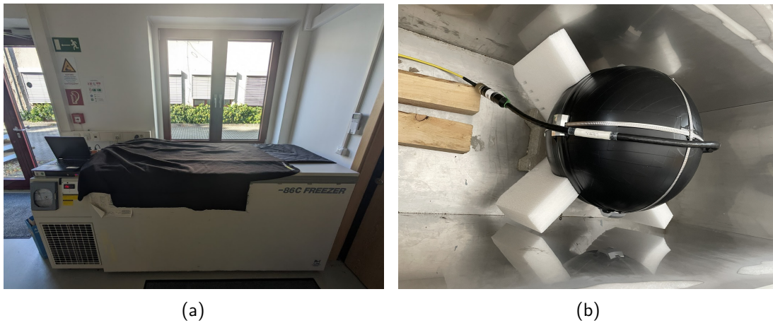
Figure 4.6: Experimental setup at DESY site for mDOM_D115_v1. Left: Freezer in which the mDOM was placed, covered by blankets. Picture by S. Blot. Right: taped mDOM inside the freezer. Picture by T. Karg.
