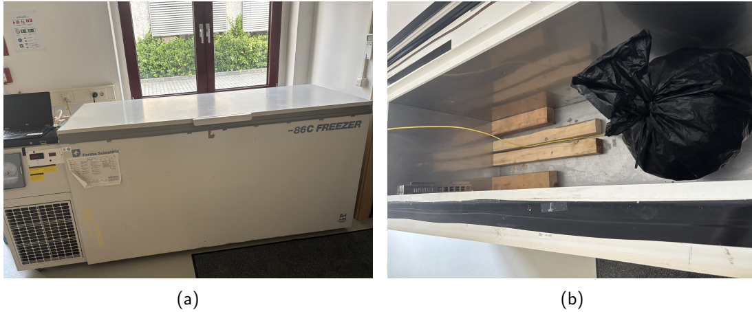
Figure 4.5: Experimental setup at DESY site for mDOM_D049_v1. Left: Freezer in which the mDOM was placed. Right: mDOM inside the freezer, covered by a black plastic bag.
