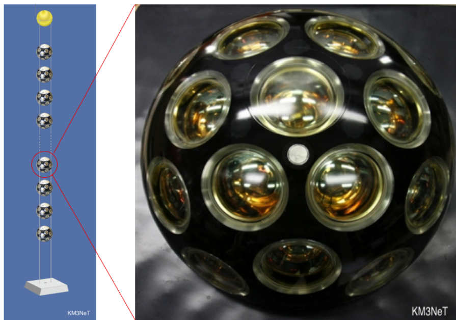
Figure 1: A close up photograph of a DOM (right). The circular cutouts are where the PMTs are positioned inside the DOM. The central white spot is the acoustic piezo sensor. Schematic view of a detection string (left), with the yellow ball at the top being the buoy.
