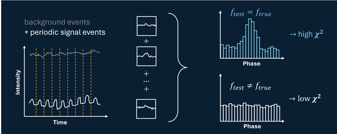
Figure 3.5: Illustration of the epoch folding algorithm. For each histogram a \chi^2 -test is performed, to check the result of the current interval choice against the background hypothesis of a flat spectrum. If a periodicity is present in the data this yields high \chi^2 values when using interval widths close to the period of the signal. Illustration made based on the examples with real data shown in [54].
