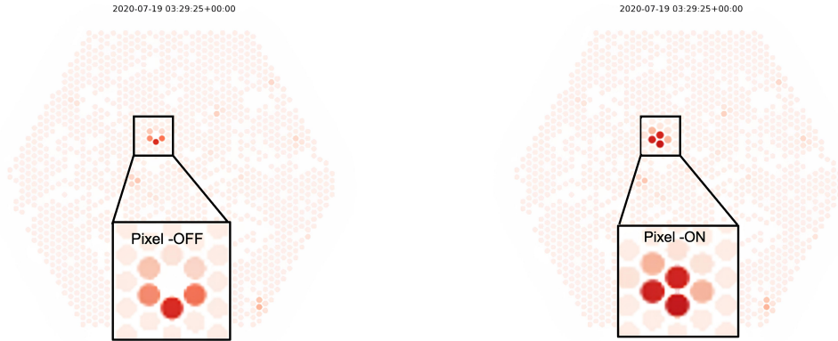
(a) “Pix-OFF”: the affected pixel is absent at this timestamp. (b) “Pix-ON”: the same pixel is present at this timestamp.
