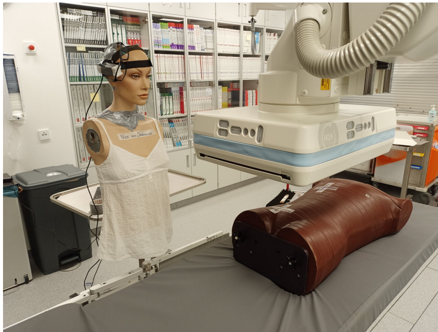
Figure 5.13.: Setup of the measurements at Marienkllinikum Siegen with additional radiation protection glasses. The eye lens dosimeter prototype is put on a plastic mannequin at different positions next to the patient table. Irradiations are performed with a medical C-arm onto an Alderson phantom.
