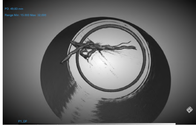
Figure 41: 3D image of the dark-field reconstruction of Sample 1. A strong dark-field signal originates from the air-cup transition and a large metal wire. This wire is a contamination of the sample and is surrounded by its strong streaking artifacts.
