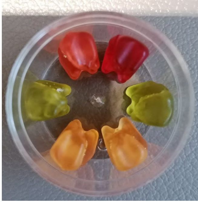
Figure 32: Plastic cup with six gummy-bears. Four gummy-bears contain aluminum-oxide powder of size d_p = 1.89 \mu\text{m} . The upper right red and green gummy-bear do not contain aluminum-oxide powder. Image taken by Markus Schneider.
