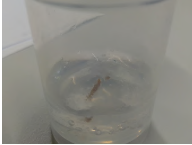
Figure 9: Gelatin phantom with three regions of different powder particle sizes and a piece of wood. The region in the front has a particle size of d_p = 24.55 \mu\text{m} , the one on the right d_p = 1.89 \mu\text{m} , and on the left d_p = 5.61 \mu\text{m} . A piece of wood is located in the middle.
