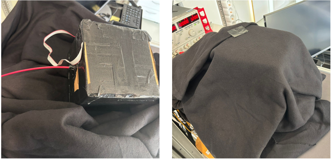
(a) The light-tight cardboard box housing the photodiode module, sealed with black tape. The ribbon cable and glass fibre exit through a small opening in the side.
