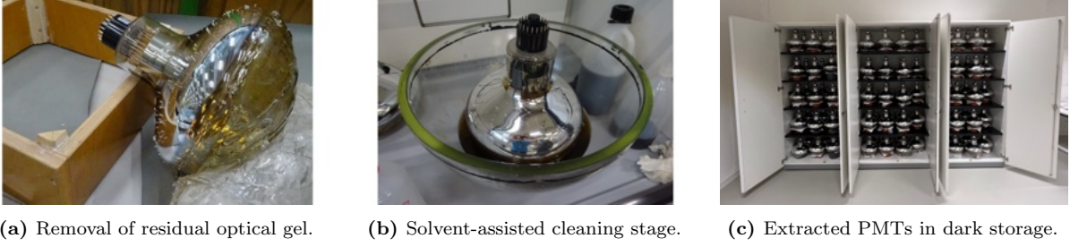
Figure 3.6: Post-release cleaning and storage of extracted ANTARES photomultipliers. Residual optical gel is removed mechanically and chemically before the recovered PMTs are transferred to dark storage. Adapted from [34].
