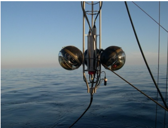
(a) Example of an ANTARES storey during deployment, showing optical modules mounted on the mechanical support structure.
