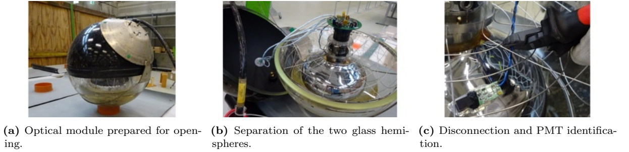
Figure 3.4: Opening sequence of an ANTARES optical module during PMT extraction. The module is mechanically opened, vented and separated into hemispheres, and the internal connections are removed while preserving PMT traceability. Adapted from [34].
