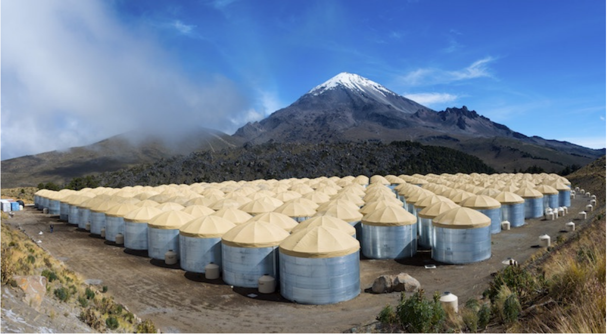
Figure 2.12: The HAWC observatory in Mexico, consisting of a dense array of water Cherenkov detector tanks.[23].
