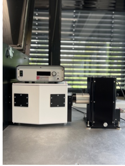
Figure 5.3: Xenon arc lamp housing used as the broadband illumination source.
