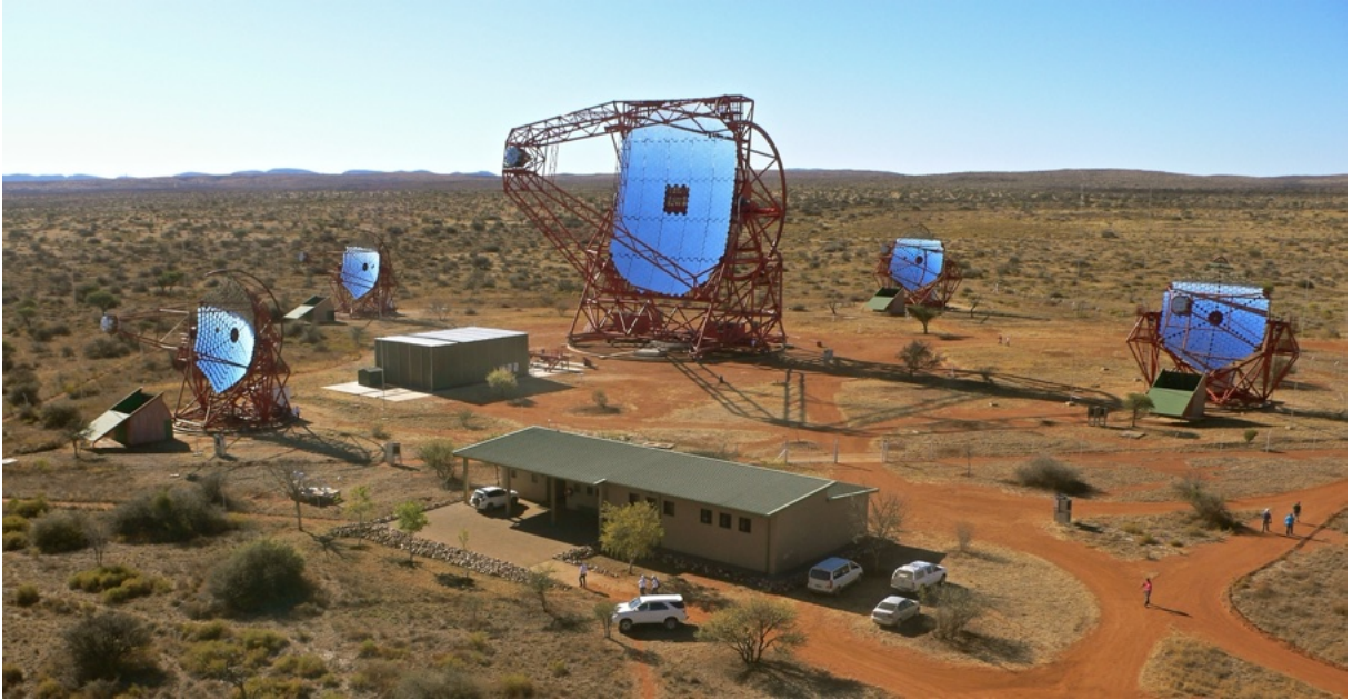
Figure 2.10: The H.E.S.S. array in Namibia, consisting of multiple imaging atmospheric Cherenkov telescopes. Arrays of this type detect Cherenkov light produced by extensive air showers and reconstruct the properties of the primary gamma ray stereoscopically. Adapted from [21].
